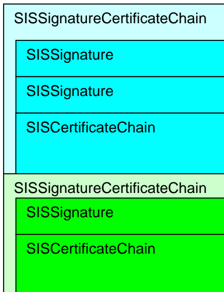
Figure 3 – Diagram of signature and certificate chain layout in SIS file
